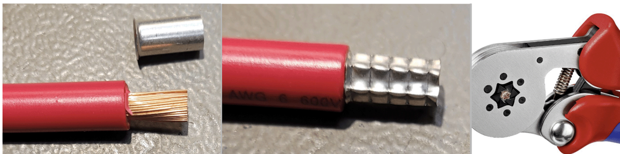
Hexagonally crimped bootlace ferrule
